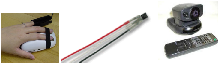
Fig. 1. GSR & BVP sensors (left), LM34 IC (center) and Eye Gaze Tracking system (right)
