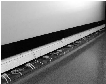
Fig. 3. 16 cameras along the floor enable object detection in front of the display wall
